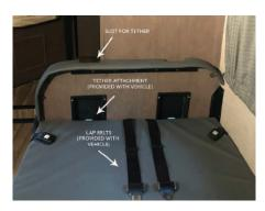
Pictures are from a C25 dinette seat, but the same on compact and large RV layout-with backrest removed showing lap belts and tethers. Depending on the size of the child, it may be necessary to fix the dinette in the lower position, i.e., bed, while traveling. For example: sometimes, the child might be too big for his legs to fit comfortably under the table; therefore, It can be an Idea to lower the table.
